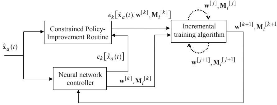
**Figure 1.6** Algorithmic diagram of constrained Policy-Improvement Routine applied to the neural network controller (1.50).
