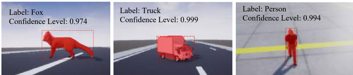
Figure 7. Examples of incursion objects simulated in UnrealEngine TM (UE). Object detection and recognition results obtained by Mask R-CNN are shown along with semantic label, bounding box, and confidence level.
