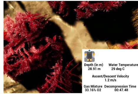
Fig. 3. Dive computer and BCD control inputs displayed on the VR interface for the real human diver
