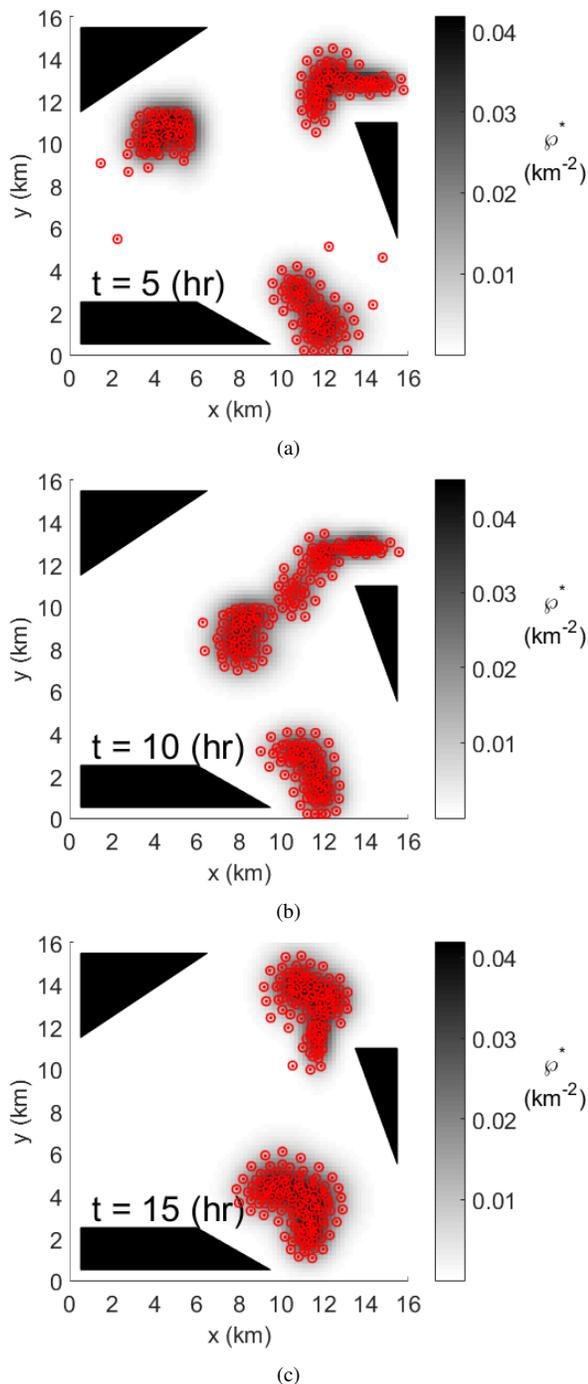
Fig. 4. Evolution of optimal sensor PDF,  $\varphi^*$ , microscopic state (red dots), and FOVs (red circles) at three instants in time
