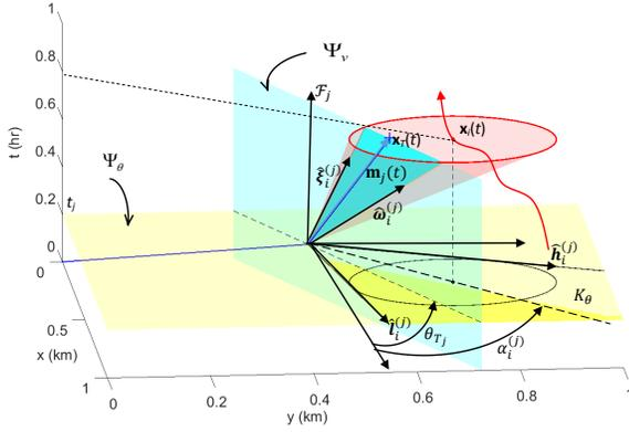
Fig. 1. Example of 3-D spatio-temporal coverage cone, where the blue curve is the trajectory of the target  $\mathbf{x}_T(t)$ . The heading-cone (yellow), velocity-cone (cyan), representation of coverage cone (magenta), and the corresponding angles are all indicated.
