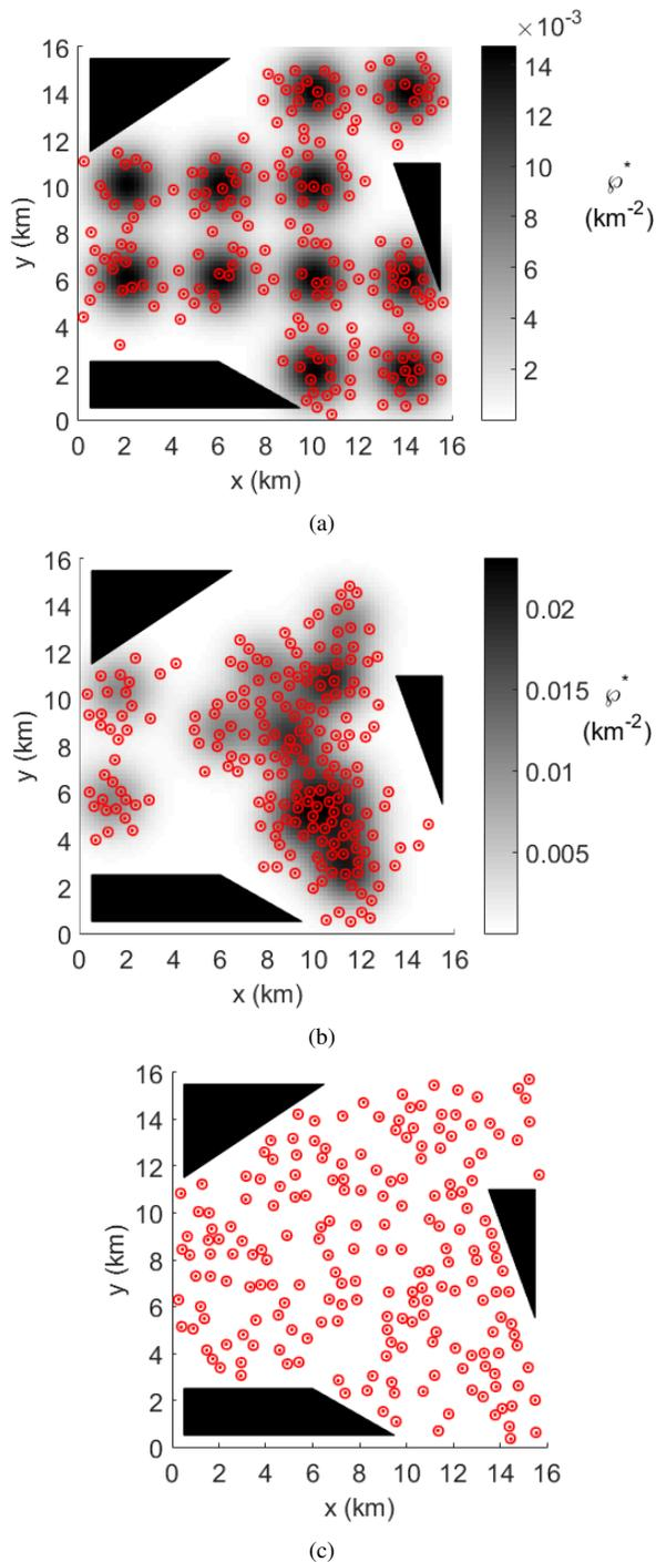
Fig. 6. Grid (a), random (b), and uniform (c) sensor deployments (red dots) and corresponding FOVs (red circles).
