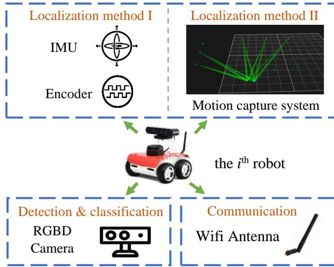
Figure 4.1: The Husarion ROSBots with various sensing capabilities.
