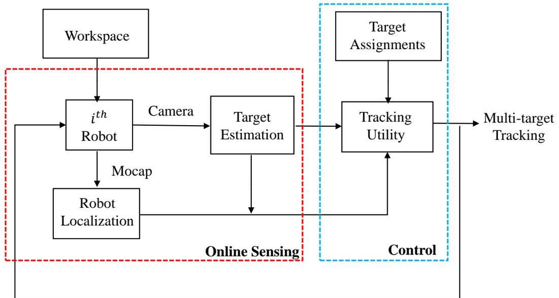
Figure 3.1: The decentralized optimization implemented on each robot.
