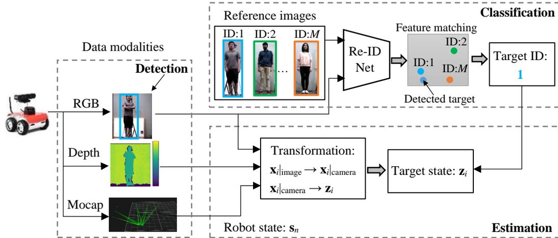
Figure 3.2: Online sensing pipeline for integrated targets detection, classification, and localization.
