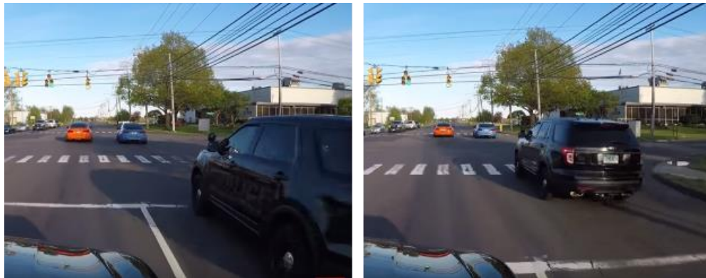
Figure 2 – Two images captured by a camera mounted on a moving car. In this scene, there are objects (other cars) that are moving independently of the car/camera. Identifying the motion of these independent objects is requires ego-motion subtraction.
