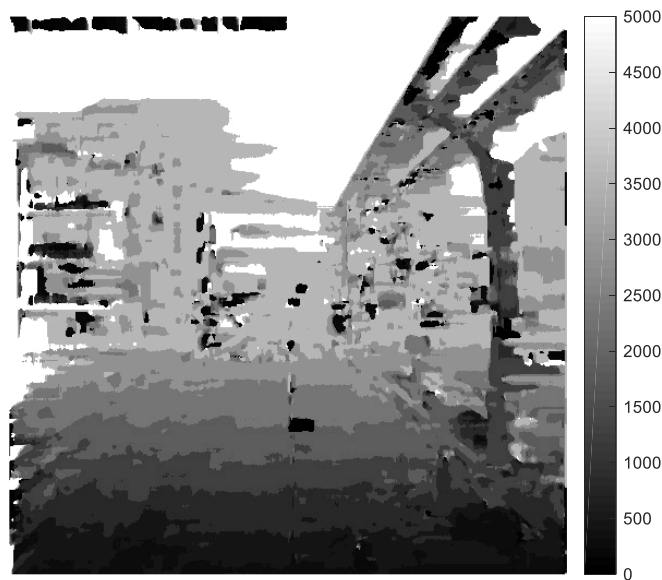
Figure 19 - Online SGM with sub-optimal convergence (to reduce computation time). The average RMSE for online SGM was 29.1%.
