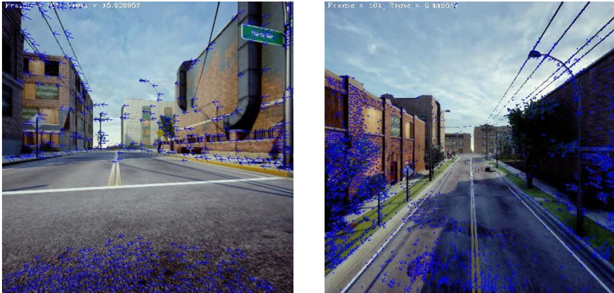
Figure 21 – Sample frames from calculating sparse (Lucas-Kanade) optical flow for camera rotation (left) and translation (right) in stationary scenes.
