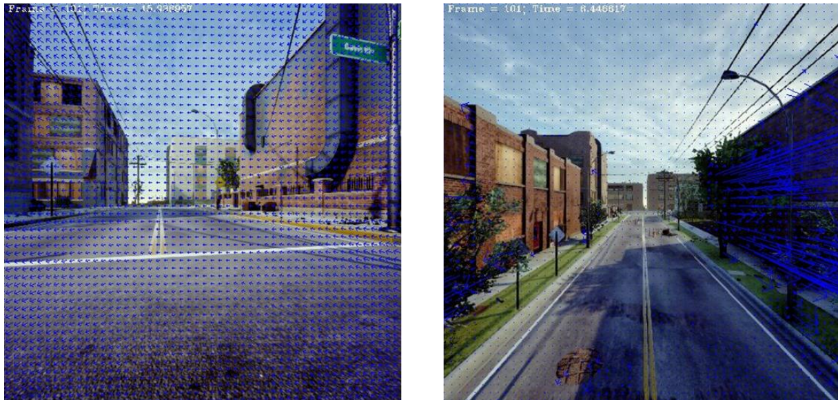
Figure 23 - Geometric Optical Flow for rotating (left) and translating (right) camera motion in stationary scenes.
