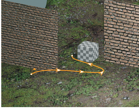
Figure 4.8: The depth estimation algorithm is applied to the data taken from the FOV of a longitudinally and laterally translating camera (shown in yellow), as it observes an otherwise static scene.
