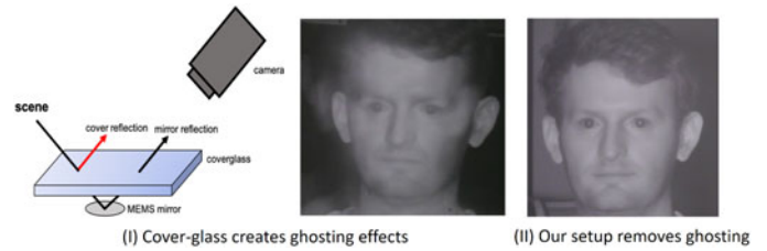
Fig. 3. The coverglass induces ghosting and double images. With a combination of using Brewster's angle, NIR notch filter and absorbing film, we eliminate the ghosting.
